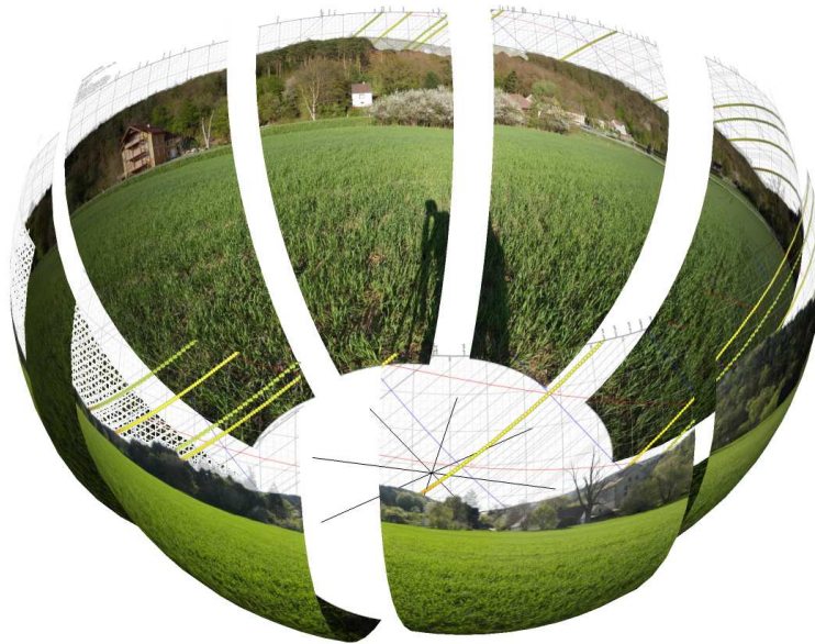
Figure 7.1: Old_style landscape: eight parts delivering a high-resolution panorama. The bottom (ground) texture, drawn on a flat plane, is not shown here.
